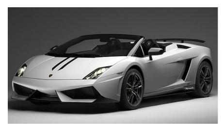
Lamborghini has announced a new, open-top, high-performance version of its Gallardo supercar, the LP 570-4 Spyder Performante. Thanks to the extensive use of carbonfibre, the new V10 sportscar has a dry weight of just 1485kg - which helps the 5.2-litre, 570HP engine to catapult the car to 62mph in 3.9 seconds. Top speed is 201 mph.
