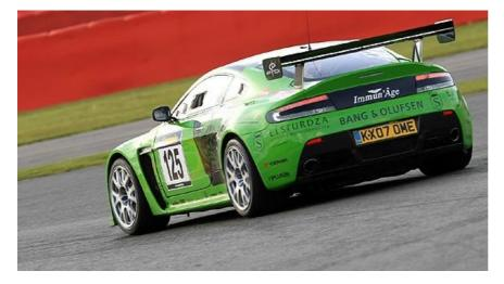
"The **Vantage** has been an experiment in what happens when you apply downforce," says **Aston engineer Paul Barritt** (the man originally behind the roadgoing **V12 Vantage**). "It has a front splitter and the rear wing, and the extractor panels behind the front wheels to draw air from under the car. The **Rapide** is as quick down the straight, but the Vantage can brake later and corner faster."
