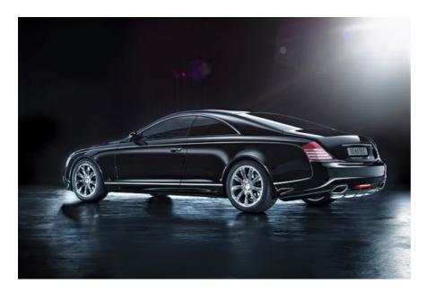
Every car will be built to individual customer specification, with wide-ranging personalisation options which can even extend to armouring the car. Changes to the 57 S base car include new doors, for easy access to the rear passenger compartment, plus a more steeply raked windscreen and rear screen to give a sportier silhouette – and to allow a lowered roofline without compromising passenger comfort.
