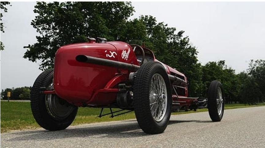
In front of me is a 2654cc version of **Jano's** double-supercharged straight eight, with heads and blocks (two groups of four cylinders) joined as one to cope with the boost pressure. Power is 215bhp, top speed is 144mph, and this car is very fit indeed.
