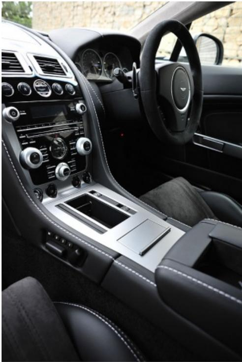
A useful feature of Aston's take on the robotised manual is that it will 'creep' in first gear, too, like a torque converter automatic.
