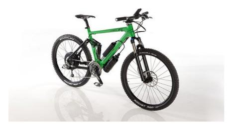
A new prototype with hybrid drive from Porsche... no, not the Cayenne S Hybrid, the 911 GT3 R Hybrid or 918 Spyder concept, but a bicycle. The Porsche Hybrid RS mountain bike weighs less than 16kg and, with electric drive assistance, has a range of more than 50km.
