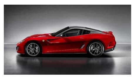
The **599 GTO** is fitted with the latest, carbon-ceramic brakes, new aerodynamic innovations such as the wheel doughnuts which increase aerodynamic efficiency as well as improve brake cooling, and 'Supersport' tyres developed by **Michelin**, with wider rubber at the front for better roadholding. Meanwhile, the **Virtual Race Engineer** (VRE) driver interface offers 'instantaneous' information on performance.
