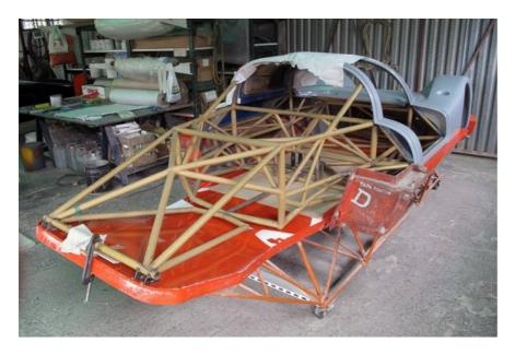
The 906 was a mid-engined car with a spaceframe chassis and a glassfibre body, all of which the Abads have reproduced with great care. The only deviation from the original specification was a deliberate strengthening of the chassis. For improved durability, they have used steel tubing of a slightly heavier gauge, making their car weigh 30kg more than the original lightweight racing car.
