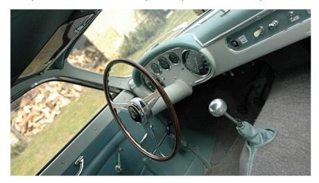
Inside, the car is beautifully trimmed in pale blue leather, with ribbed headlining (also in leather) that complements the pale grey exterior. **Zagato** is well-known for its lightweight construction, so you will see wind-up Perspex windows in fabricated, natural aluminium surrounds. Even the winders are alloy, with tiny hinged ends that fold out of harm's way.
