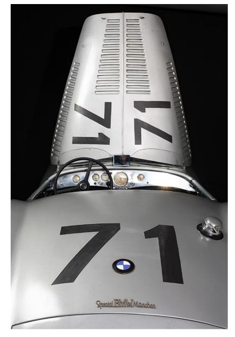
The unique bodywork of the re-engineered car became the pattern for a whole generation of post-War sports cars, and clearly influenced such models as the **Jaguar XK120 Roadster**. Among the other modifications was an intricate tubular steel framework, while key components such as brakes and the **Hurth** gearbox were uprated to cope with the increased performance of the 130PS engine and lighter kerb weight of 725kg.
