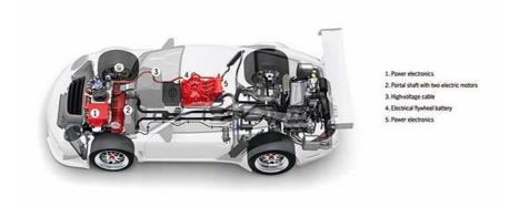
On the face of it, it would appear to be similar to the ill-fated 'KERS' system in Formula One. The flywheel is located next to the driver for optimum weight distribution. As a result of the new system saving energy, the 'rolling laboratory' will be more fuel efficient, too – vital in a 24-hour race.
