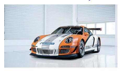
This is a hybrid version of a racing 911 which features two electric motors driving the front wheels, in addition to a conventional 4.0-litre, 480bhp flat-six/rear-wheel drive configuration in the back. The car will be launched at Geneva and make its racing debut in Nürburgring long-distance events, including the 24 Hours meeting on May 15-16 2010.
