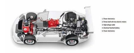
On the face of it, it would appear to be similar to the ill-fated 'KERS' system in Formula One. The flywheel is located next to the driver for optimum weight distribution. As a result of the new system saving energy, the 'rolling laboratory' will be more fuel efficient, too – vital in a 24-hour race.
