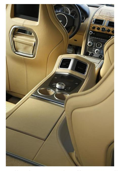
As a driver or front-seat passenger in a **Rapide**, **DB9-owners** would notice the extra width of the all-new **Recaro** seats and a general feeling of spaciousness. This is achieved by an electronic handbrake replacing the fly-off, and much bigger rear side-windows allowing more light into the cabin.
