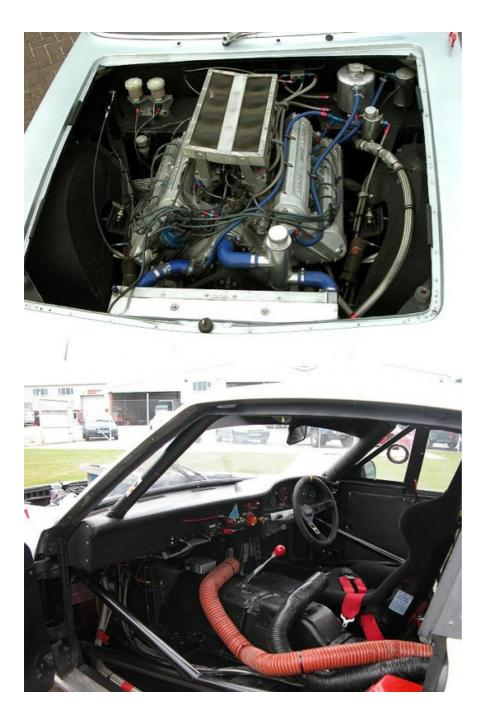
The dry-sumped V8 was completely overhauled in 2007, completing just 14 racing hours since then. Braking is courtesy of a six-pot **Automotive Products** (AP) system and **AP** floor-mounted pedal 'box.
