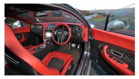
The carbonfibre, 'clam shell' **Sparco** bucket seats in the front are brilliant. Beautifully trimmed in leather and **Alcantara** at **Crewe**, with just fore-and-aft plus backrest manual adjustment, these provide one of the most comfortable driving positions I've experienced. It's a classic case of 'less is more'; get the position spoton to start with and you can dump the weighty electric adjustment for good.
