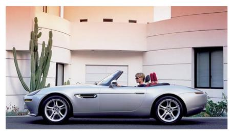
No less than six feet wide between its chrome-embellished mirrors, it weighed in at 1585kg, making it 180kg lighter than the contemporary **M5** which shared the same 394bhp, 4941cc V8 engine. That produced a stunning 0-60mph time of under five seconds for the **Z8**, and a top speed of over 160mph.
