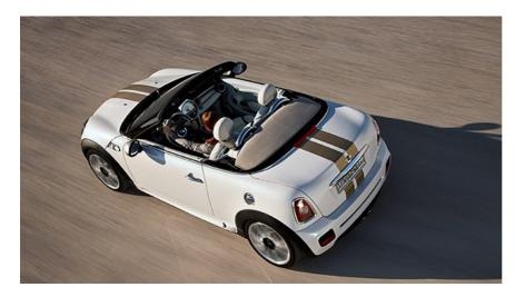
The soft top opens and closes manually, with the emphasis on low weight and compact dimensions, folding down to sit on top of the rear luggage compartment – and hence there's no reduction in bootspace with the roof down. There is access to the luggage compartment from the cabin, via a lockable opening in the bulkhead.
