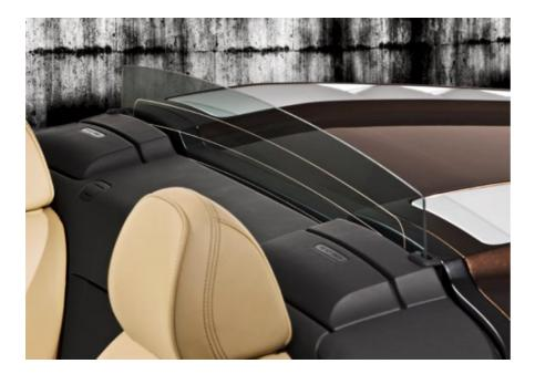
The electrohydraulically controlled roof opens and closes in 19 seconds at speeds of up to 31mph. Separate from the fabric roof is a heated glass window, which can be raised and lowered (into the bulkhead) at the touch of a button, with the roof up or down.
