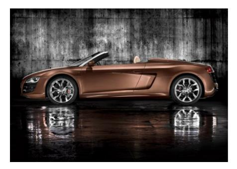
The weight of the open-topped car is minimised by Audi's (fully automatic) lightweight fabric roof – just 30kg – as well as the aluminium spaceframe and carbonfibre composite panels of the body.
