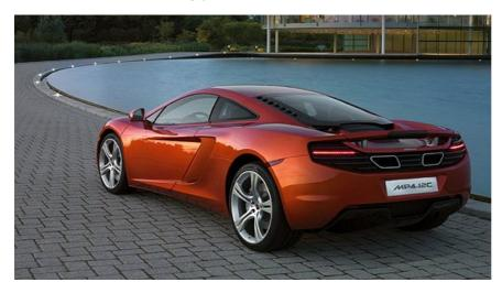
Cast alloy wheels (19in front, 20in rear) are fitted with **Pirelli** tyres specially developed for the MP4-12C. Brakes, unusually, are steel with forged aluminium bells as standard. Carbon composite discs will be an option, but are heavier than steel and therefore go against the extreme weight-saving ethos of the new car. Additional braking at very high speed is provided by the moveable rear airbrake.
