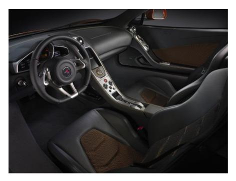
The functional but beautifully finished interior contains no parts from other cars; every component is special to the MP4-12C. Like the original **McLaren F1**, many controls have been moved to the most ergonomic positions, such as the armrests of the doors.
