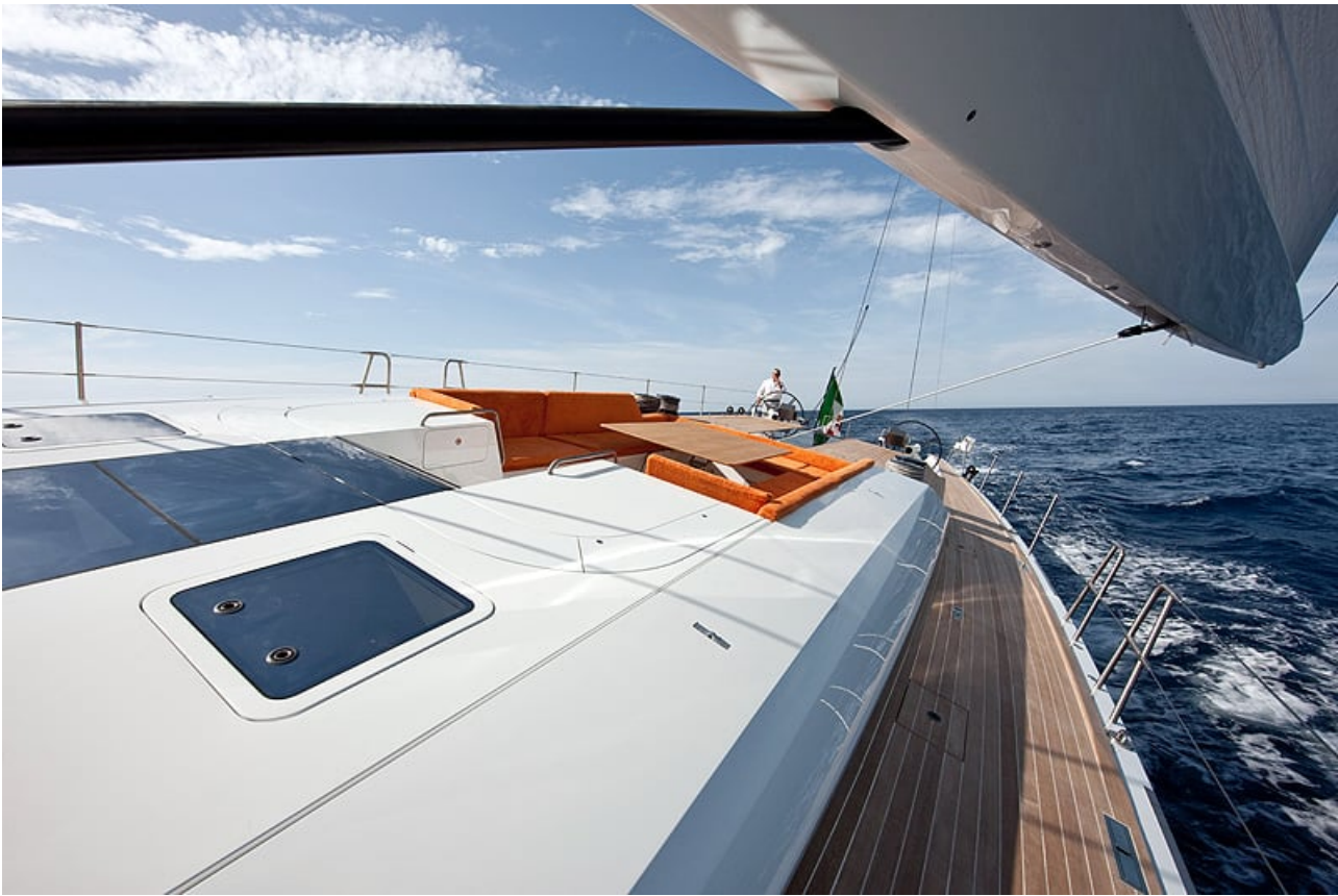
The new Wally 101 is a further development of the 100-footer Y3K. The mast is made from light but sturdy carbon composite, with sails that have a maximum area, when sailing downwind, of 1259sqm.
