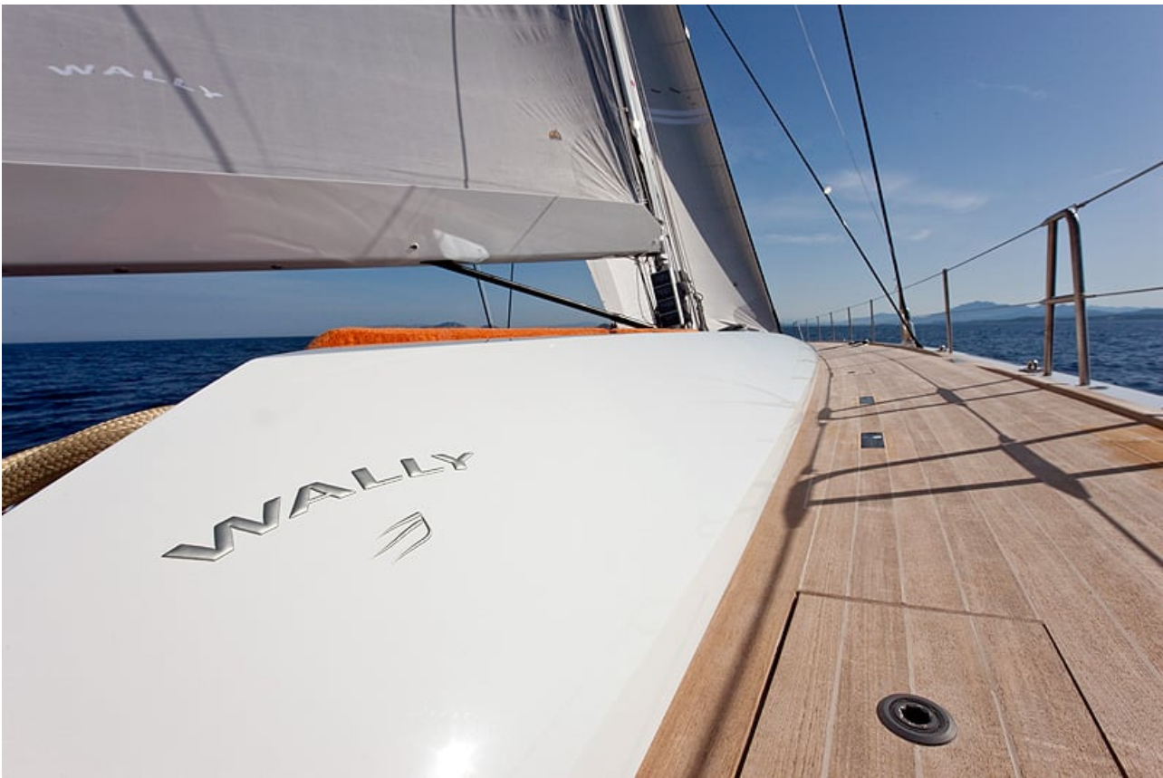
The new Wally 101 is a further development of the 100-footer Y3K. The mast is made from light but sturdy carbon composite, with sails that have a maximum area, when sailing downwind, of 1259sqm.
