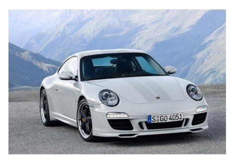
Power from Porsche's 3.8-litre engine has been upped by 20HP to give 408HP, through the introduction of a newly developed resonance intake manifold with six vacuum-controlled switching flaps. The 911 Sport Classic comes with a six-speed manual gearbox, PCCB Porsche Ceramic Composite Brakes, PASM sports suspension (lowering the car by 20mm), and custom-made 19-inch wheels with black-painted rim stars.
