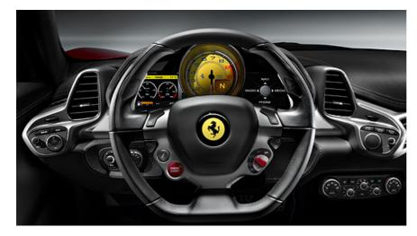
The right-hand satellite pod incorporates controls for the infotainment, the Bluetooth connection, sat-nav, digital speedo and rear parking camera. In the left-hand pod are the (optional) cruise control and the onboard computer interface. The latter controls the trip computer, **Vehicle Dynamic Assistance** and the display of the car's set-up.
