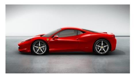
Using a combination of advanced aluminium alloys, with aerospace industry bonding techniques, Ferrari engineers have kept the dry weight down to 1380kg, 58 per cent of which is over the rear axle. This has enabled 0-62mph acceleration in under 3.4 seconds. Top speed is over 202mph.
