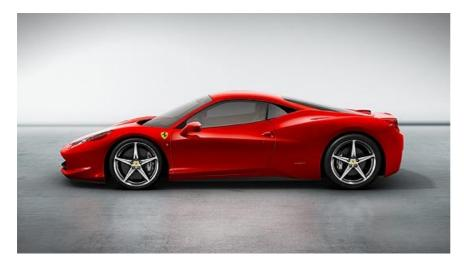
Using a combination of advanced aluminium alloys, with aerospace industry bonding techniques, Ferrari engineers have kept the dry weight down to 1380kg, 58 per cent of which is over the rear axle. This has enabled 0-62mph acceleration in under 3.4 seconds. Top speed is over 202mph.
