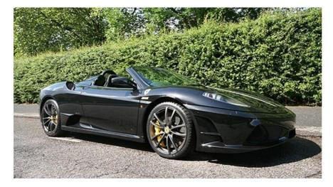
The extensive use of carbonfibre and stripped trim has taken 80kg off the weight of the F430 Spider, reducing the Scuderia 16M down to 1340kg. The 16M features, as standard, the rear carbon diffuser panel which was a £10k option on the Scuderia Coupé.
