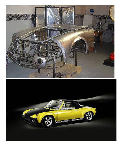
Automotive projects include making the one-off coachwork for an **Aston Martin V8 Vantage Shooting Brake**, the complete restoration of an **Alfa Romeo Giulietta SZ** *Coda Tronca*, a **Porsche 914/6 GT** and a rare, all-aluminium **Mercedes-Benz 300 SL Gullwing**.
