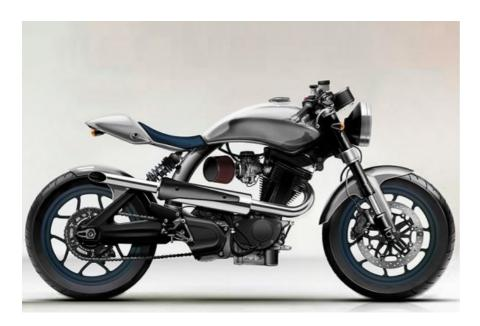
Mac motorcycles are built simply and powered simply – the small range of lightweight, air-cooled singles uses the 500cc Buell 'Blast' motor in a tubular backbone frame.
