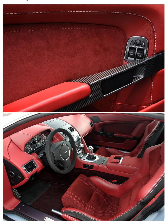
Inside, the cabin is to Aston's regular 2009-spec with only simple changes that include: lightweight carpet, an Alcantara-covered steering wheel and carbonfibre door pulls. Sat-nav is standard, as is the Emotional Control Unit crystal key. Hats off to the Gaydon team for resisting the temptation for in-car timing, a roll-cage or six-point harness.
