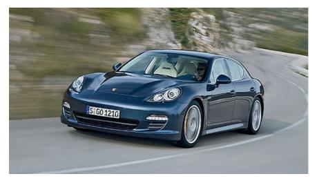
Meanwhile, the chassis and suspension of the Panamera aim for a high standard of comfort but – at the touch of a button on the active PASM damper system – the settings switch to a fully sports suspension. Adaptive air suspension with 'extra volume' when required – a refreshingly new idea – comes as standard on the Turbo and an option on the other models.
