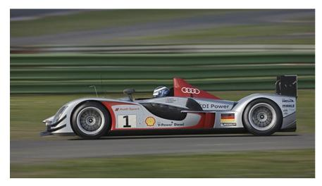
The 12-hour race at Sebring will also be the debut for the new technical regulations for Le Mans prototypes. Diesel-powered cars must compete with smaller air-intakes and lower turbo pressure – hence less power – while the width of the rear wing has been reduced by 40cm.
