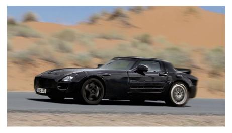
The aluminium spaceframe body will have – gulp – gullwing doors, with an AMG 6.3-litre V8 front-midmounted engine developing 563bhp. Other technical details so far released include dry-sump lubrication, seven-speed dual-clutch transmission and aluminium double-wishbone suspension. Meanwhile, Mercedes is promising front/rear weight distribution of 48:52 – with, of course, a satsifyingly low centre of gravity.
