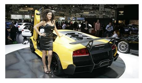
Visually – rear tea-trays apart – the latest iteration of the company's flagship has new air management treatment at the front, with matt black-painted parts mixed with carbonfibre. The engine is visible under hexagonal polymer plates made from transparent polycarbonate, set on three levels within a carbonfibre framework.
