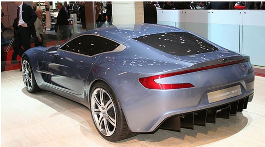
The car is likely to weigh in at 1500kg, will wear unique-to-the-car Pirelli P Zero Corsa tyres (255/35 ZR20 front, 335/30 ZR20 rear), and will transmit its 700+bhp to the road through the rear wheels, via a new six-speed gearbox. The gearbox uses the principles of the company's Sportshift transmission, but is heavily uprated to cope with the extra power and torque. CCM brakes are standard.
