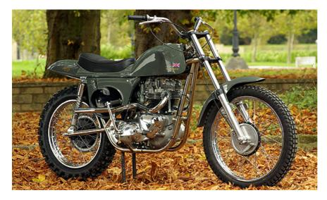
The bikes include styled footrests made to the original design and 35mm Ceriani forks with seven inches of travel, which McQueen found to be optimal. The yokes are from BSA – his preference, due to the handlebar position, set behind the steering stem for better control. Complete bikes are ready to order now, utilising a fully reconditioned period Triumph engine, complete with a single Amal carburettor. The price is £12,999, excluding VAT.
