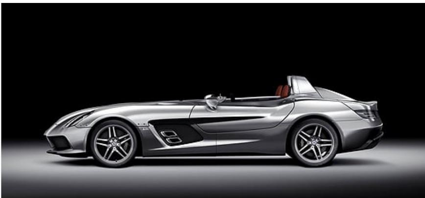
The two-seater has neither roof, nor side- or front-windows, with small air deflectors on the arrow-shaped bonnet to keep the bugs out. Removable tonneau covers are kept in the boot and provide all-weather protection and, like the 1950s Le Mans car, the car is equipped with an AIRBRAKE.
