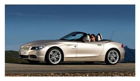
In what is a first for a BMW roadster, the new Z4 - due to go on sale in the UK in May - has a retractable metal roof. The two-piece electrohydraulically operated hard-top, which opens or closes in 20 seconds, is just one in a number of innovations for the all-new model.
