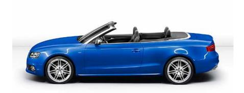
The initial engine line-up will be two FSI direct injection petrol engines and one TDI diesel: 2.0 TFSI (211PS), 3.2 FSI (265PS), 3.0 TDI (240PS). The diesel will come with quattro as standard, but 4wd will also be offered across the range as an option. Transmissions are either 6-speed manual, an 'S tronic' twin-clutch 7-speed automatic or 'multitronic' CVT. S tronic is only available on the 3.0 TDI quattro and is standard on the range-topping S5 Cabriolet.
