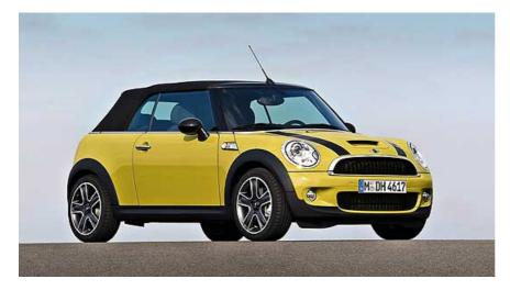
The roof of the new model opens and closes via a toggle switch in 15 seconds and can be operated at speeds up to 20mph. Alternatively, the roof can be electrically retracted by about 40cm, sunroof-style, at up to 75mph.
