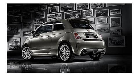
The car has all the performance addenda no self-respecting Abarth would be without: ventilated disc brakes front and rear; high-performance front brake pads; special lowered springs and 17in alloy wheels fitted with Pirelli P Zero Nero 205/40 R16 ZR 17 tyres and, a – unique to the car – four-pipe exhaust.
