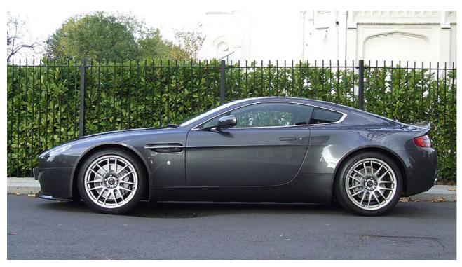
Far from turning the V8 Vantage into a harsh car suited only to track-day use, however, the suspension modifications – with driver switchable damper mode – are actually intended to improve the ride quality of the standard car, particularly over bumps and compressions. And when combined with Prodrive's 19in forged aluminium wheels of 8.5in and 10in width, clad in Pirelli P Zero Corsa tyres, there is a perceptible increase in grip.
