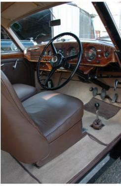
The wheel is large but well-suits the combination of tall cross-ply tyres and cam-and-roller steering box. The driver sits relatively tall 'in the saddle', surveying the exquisite marquetry of the dashboard, typical period instrumentation (to which Rolls-Royce and Bentley still pay homage) and the flying 'B' some distance away, atop the chrome radiator shell.
