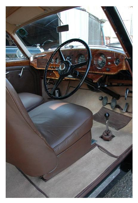
The wheel is large but well-suits the combination of tall cross-ply tyres and cam-and-roller steering box. The driver sits relatively tall 'in the saddle', surveying the exquisite marquetry of the dashboard, typical period instrumentation (to which Rolls-Royce and Bentley still pay homage) and the flying 'B' some distance away, atop the chrome radiator shell.
