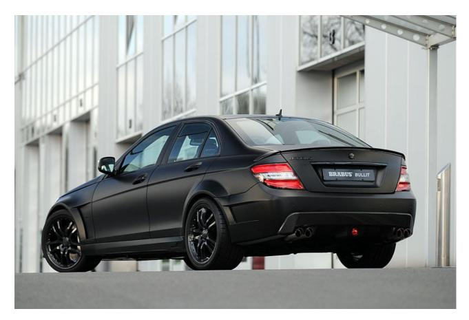
Behind the flared wheelarches, the 9.5Jx19 front wheels are shod with 265/30 ZR 19 tyres, while the 10Jx19 rears wear size 285/30 ZR 19. To stop them turning, the Brabus brake system boasts 12-piston aluminium fixed calipers at the front, gripping 380mm vented and grooved discs. At the rear, six-piston calipers work on 360mm discs.
