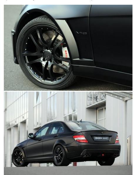
Behind the flared wheelarches, the 9.5Jx19 front wheels are shod with 265/30 ZR 19 tyres, while the 10Jx19 rears wear size 285/30 ZR 19. To stop them turning, the Brabus brake system boasts 12-piston aluminium fixed calipers at the front, gripping 380mm vented and grooved discs. At the rear, six-piston calipers work on 360mm discs.
