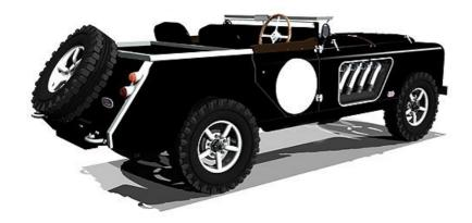
Under the never-ending bonnet lies a choice of 8- or 12-cylinder 4.6-litre engine, while the passenger compartment is appropriately minimalist and the traditional leaf spring chassis transmits every detail of the road surface through to the driver's spine. The Longnose features the unsurpassed off-road capabilities of an authentic Land Rover, with four-wheel drive, off-road gear reduction and central locking differential.
