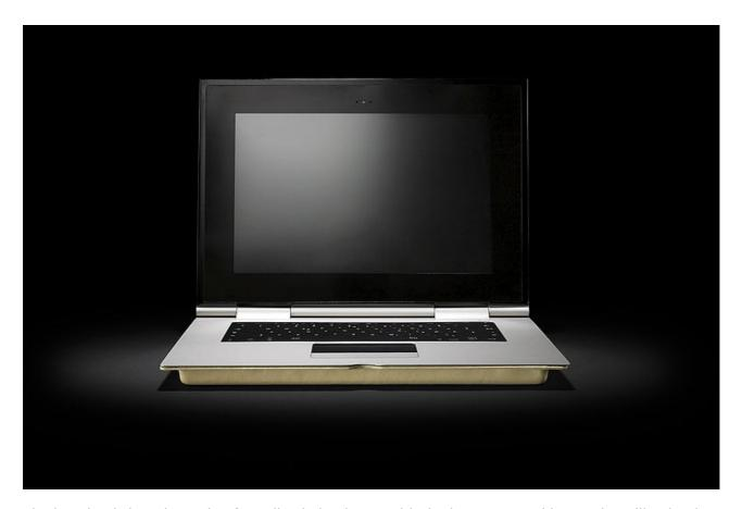
The housing is largely made of anodised aluminum, with the base encased in supple aniline leather, available in a choice of black, ivory or dark red. The use of fine leather extends to the two calf-leather carrying cases supplied with each Workstation.
