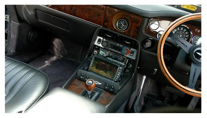
Fitted in the boot is componentry to power the state-of-the-art Alpine Sat-Nav/DVD/TV system. Twin screens (front and rear) can keep the occupants in the rear updated with the latest news from Wall (or Ramsay...) Street, while up front the driver won't miss a turning, thanks to the satellite navigation nestling just forward of the gearlever.
