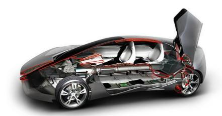
Pininfarina has extended its innovation to the whole four-door sports car concept. Instead of viewing the body as a covering for the engine and associated technologies, Pininfarina has adopted a policy it calls 'Liquid Packaging', shaping the technology around the passengers, improving weight distribution and lowering the centre of gravity.
