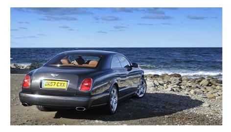
The flawless paint finish is matched by all-stainless steel external brightware, and the bodywork – 130 hours of hand-construction that includes copper-brazed joints, 6000 hand spot welds and 15m of seam welding – personifies the coachbuilder's craft. It's big and, with the exception of just a slight excess in height towards the rear of the roof, works very well.
