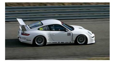
Several suspension components for the GT3 Cup S have been taken from the more powerful GT3 RSR, and its braking system has been upgraded with 5mm larger diameter discs at the rear (to 355mm).
