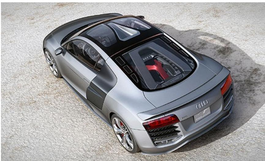
The diesel engine itself is displayed in all its glory beneath a clear glass cover. At 684mm in length, the 12-cylinder is 166mm longer than the V8 TDI. It doesn't sound a lot but I can't imagine it was an easy job to squeeze it into the engine bay. Audi says that the sensation of space which sets the R8 apart from rivals is 'barely' compromised. Whatever that means.
