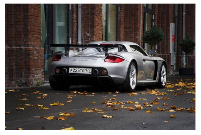
There are also mods to the aerodynamics, with an edo competition rear wing fabricated entirely from carbonfibre. The centre portion of the Gurney flap rises, along with the retractable rear wing, to produce additional downforce on the rear axle – plus there are fixed flaps on either side of the wing.
