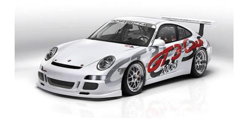
Porsche is updating its 911 GT3 Cup race car, based on the road-going GT3, for the 2008 motorsport season. Power from the 3.6-litre six-cylinder boxer engine will increase by 20bhp to 420bhp, and there will be significant changes to the rear end along the lines of the production model's design, with air-venting slits to dissipate heat more effectively.
