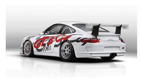
The 26 units built for the Porsche Mobil1 Supercup feature a special exhaust system with an even more striking sound, "reminiscent of the Formula 1 racing scene". They also have PCCB Porsche Ceramic Composite Brakes. The race cars entered worldwide in the Carrera Cup, meanwhile, will feature a modified exhaust system and steel brake discs.
