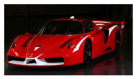
Maranello's engineers studied the wealth of information gained to develop a kit which will cut the FXX's Fiorano lap time to under 1min 16sec – a substantial two-second improvement. The FXX's 6262cc V12 engine can now punch out a massive 860hp at 9500rpm, while gearshifts take just 60ms, a drop of 20ms on the previous time, and the gear ratios have been adapted to make use of the extra 1000rpm now delivered by the engine.
